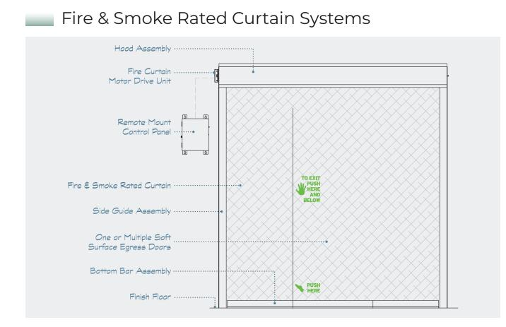
The McKEON D200E side guide configuration, with a maximum of a 1/2" reveal, can be surface or flush mounted making it virtually invisible in any application.
